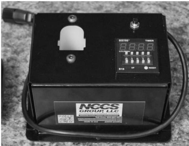
8. Plug the Rechargeable Battery into the Power Box battery hole. DO NOT apply much force. When the Rechargeable Battery is properly connected, the Timer will turn on.
