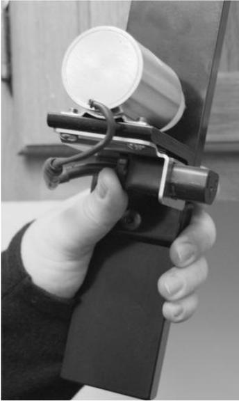
10. With right hand insert the Power Cord into the Plug on the Stabilizer Arm.
