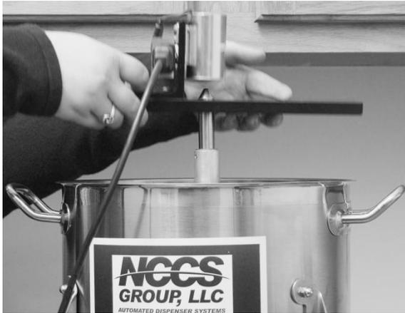
12. Pour the liquid into the Juice Container in the opening opposite of the Power Cord making sure that no liquid is poured over the Stabilizer Arm. Fill until the liquid is within the Fill Range, between the top and bottom screws. As covered in *Setting the Timer* on pages 32-34, the amount of liquid in the Juice Container controls the rate of the flow of liquid. Keep the liquid level between the top and bottom screws while the System is in use.
